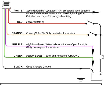
These lights are standard **negative ground**. Isolated or floating units for positive ground vehicles are clearly labeled and are available upon request. In this case connect the power to the proper polarity as marked on the wires.
